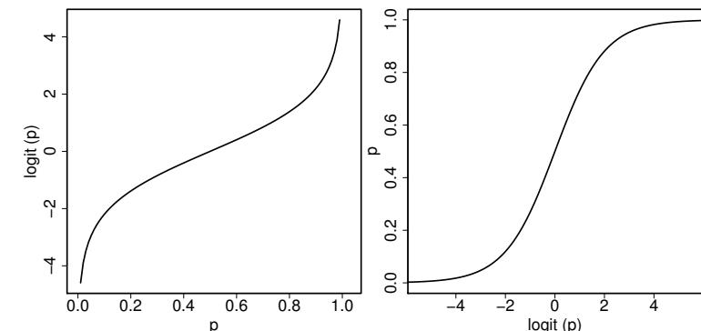
$$p_i = \frac{\exp(\alpha + \beta_1 x_{i1} + \dots + \beta_d x_{id})}{1 + \exp(\alpha + \beta_1 x_{i1} + \dots + \beta_d x_{id})}. \quad (4)$$
